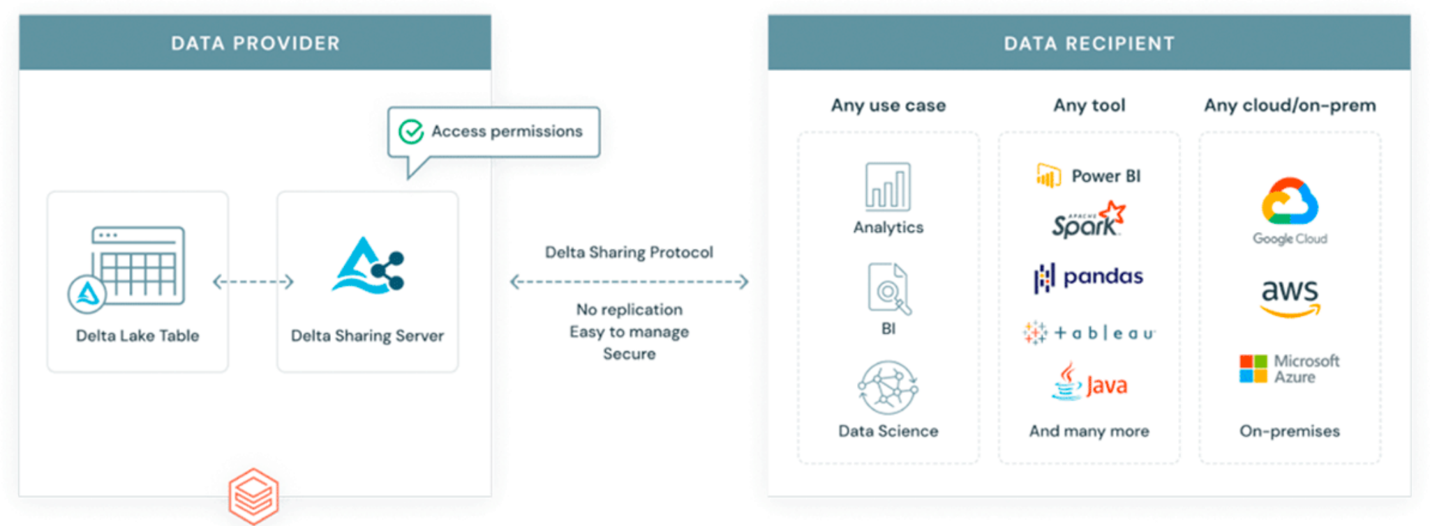
Figure 7: Delta Sharing simplifying data access in the ecosystem
